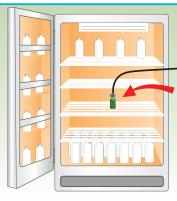
Place the buffered probe in the center of the refrigerator near the
